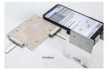
Fig. 1. The 2D Measuring System MICRO CONTROL consisting of a Smartphone, Measurement tools and the PointArea
